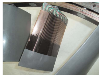
Fig. 4 Compressor blade instrumented with an array of hot-film sensors
